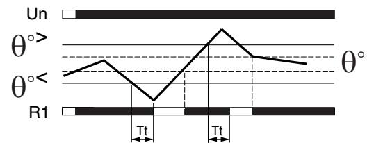
T<sub>t</sub> : time delay on opening, after temperature threshold overshoot (adjustable on front panel)
