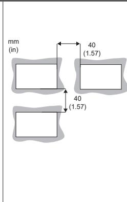
**en** Minimum clearance between flush mounted devices
