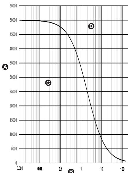
**en** Resistance vs system capacitance graph for the device threshold values.
