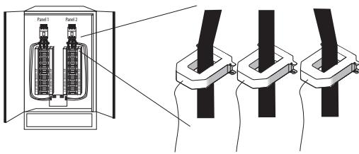
**en** Mains CTs: Use CTs with 0.333 Vac outputs, LVCT Series recommended. Install on main feeds according to instructions provided with CT. If the signed power factor feature is enabled, the sensors must be oriented so that the arrow points toward the load for proper operation.
