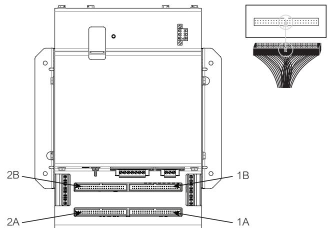
**en** If the signed power factor feature is enabled, the sensors must be oriented so that the arrow points toward the load for proper operation. Connect the black and white lead wires from each branch CT to the corresponding terminals on the adapter board. There is a row of terminals for the black wires and a row of terminals for the white wires.
