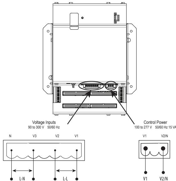
**en** For voltage inputs V1-V3: L-L voltage: 150 to 480 Vac, nominal, L-N voltage: 90 to 300 Vac. Voltage taps are shared by both panels
