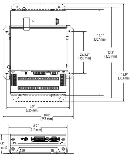
**en** Dotted lines indicate dimensions if the two brackets are placed for horizontal mounting. At the factory, the brackets are placed for vertical mounting.
