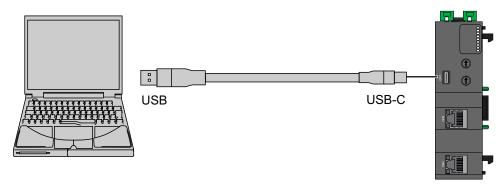
The communication cable should be connected to the PC first to help minimize the possibility of electrostatic discharge affecting the network interface module.
