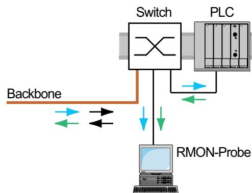
On the destination port, the device only forwards the data packets copied from the source ports.
