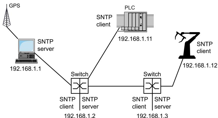
**NOTE:** For precise time distribution, between SNTP servers and SNTP clients you preferably use network components (routers and switches) that forward the SNTP packets with a low and uniform transmission time (latency).
