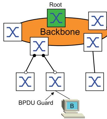
Terminal device ports do not normally receive any STP-BPDUs. If an attacker still attempts to feed in STP-BPDUs on this port, then the device deactivates the device port.
