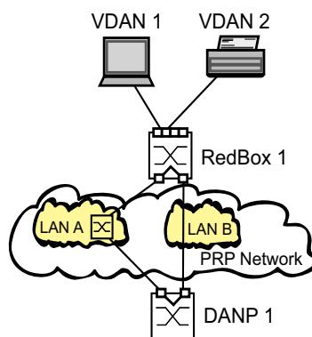
**NOTE:** **PRP** is available for devices with an FPGA (hardware for extended functions). The product code indicates if your device supports **PRP**. To use the functions, load the device software supporting **PRP**.
