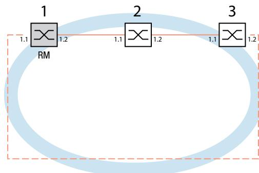
The following example configuration describes the configuration of the Ring Manager device (1). You configure the 2 other devices (2 to 3) in the same way, but without activating the *Ring manager* function. This example does not use a VLAN. You specify the value *30ms* as the ring recovery time. Every device supports the advanced mode of the Ring Manager.
