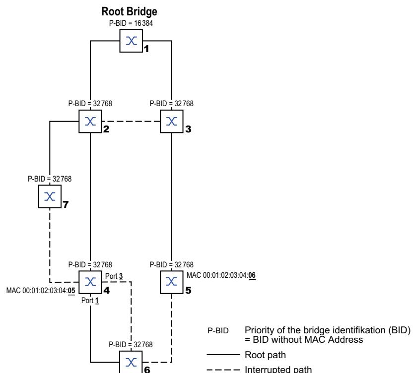
**NOTE:** When the present root bridge goes down, the MAC address in the bridge identifier alone determines which bridge becomes the new root bridge, because the Administrator does not change the default values for the priorities of the bridges in the bridge identifier, apart from the value for the root bridge.
