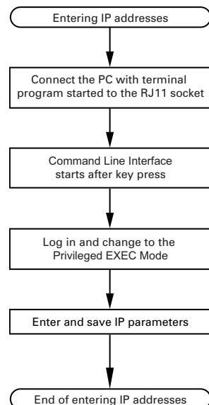
**NOTE:** If a terminal or PC with terminal emulation is unavailable in the vicinity of the installation location, you can configure the device at your own workstation, then take it to its final installation location.
