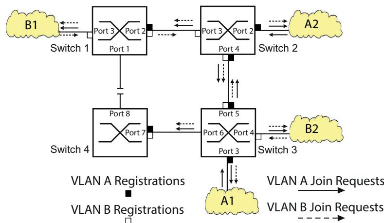
In the MVRP example network, the LANs first send a Join request to the switches. The switch enters the VLAN registration in the forwarding database for the port receiving the frames.
