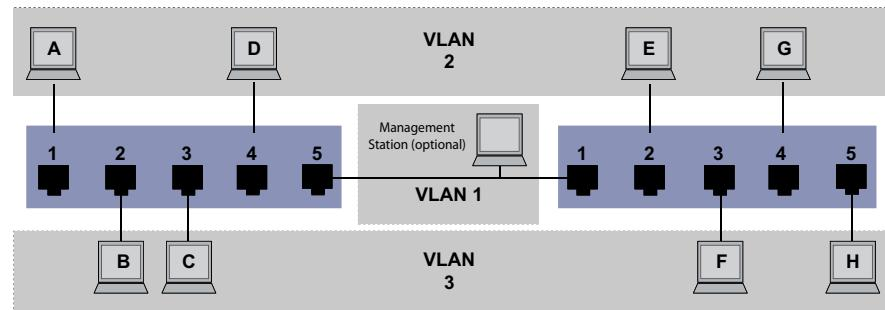
The terminal devices of the individual VLANs (A to H) are spread over 2 transmission devices (Switches). Such VLANs are therefore known as distributed VLANs. If the VLAN is configured correctly, then an optional network management station is also shown, which enables access to every network component.
