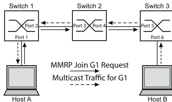
Enable the **MMRP** function on the switches. To do this, perform the following steps:
