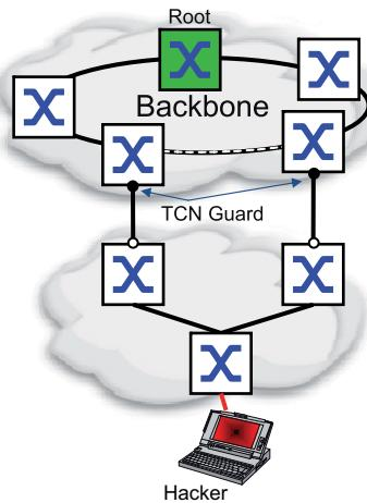
If the protection function is activated, then the device ignores Topology Change flags in received STP-BPDUs. This does not change the content of the address table (FDB) of the device port. However, additional information in the BPDU that changes the topology is processed by the device.
