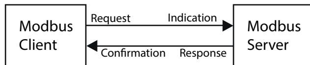
The client / server model uses four types of messages to exchange data between the client and server:
