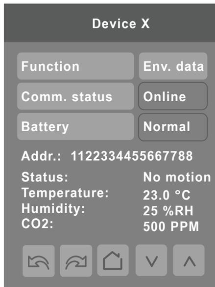
8. After the sensor has paired with Room Controller, make sure the **Function** parameter matches the Zigbee sensor type, and if required change it accordingly to one of the following choices:
