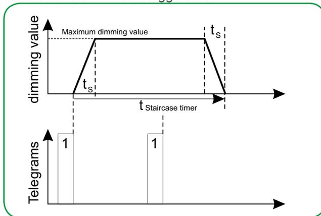
However, if the staircase lighting time is not retriggerable, the output will switch off/dim at exactly the moment the time elapses. If the *Manual switching off* function is activated, the staircase lighting time can be terminated prematurely with a "0" telegram.
