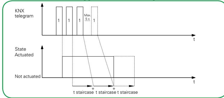
Once one or more new telegrams with the object value “1” have been received, the staircase lighting time is added to the previous staircase lighting time. The number of additions can be set. You can parameterize a maximum of 5 additions of the staircase lighting time. For example, you can add up the staircase lighting time by pressing a separate button several times.
