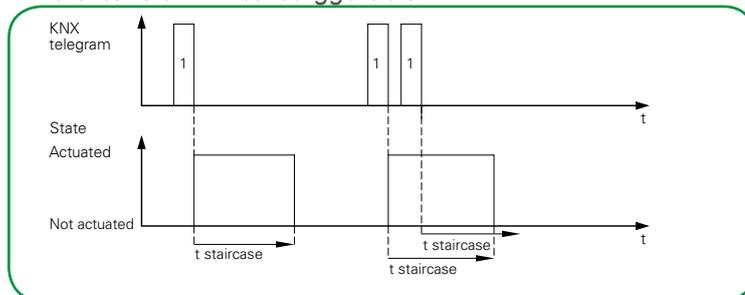
However, if the staircase lighting time is not retriggerable, the relay will switch off at exactly the moment the time elapses. If the *Manual switching off* function is activated, the staircase timer can be ended with a “0” telegram.
