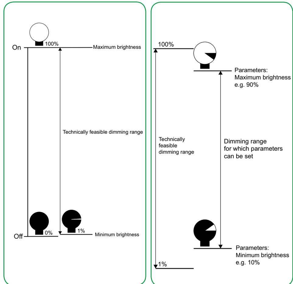
The dimming range can be limited further using the software application. This limit can be set individually for each output channel.
