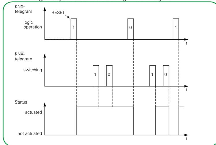
The logic object is preset to the value “1” after a RESET. The actuator will switch on the output immediately. The OR logic function is only reset by a “0” telegram on the logic object.
