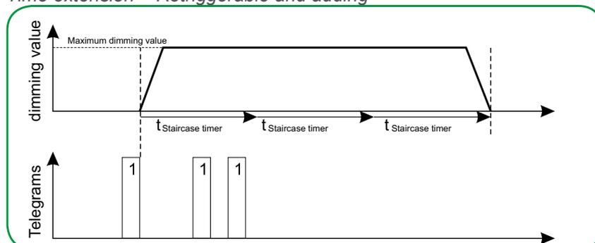
Once one or more new telegrams with the object value "1" have been received, the staircase lighting time is added to the previous staircase lighting time. The number of additions can be set. You can parameterize a maximum of 5 additions of the staircase lighting time. For example, you can add up the staircase lighting time by pressing a separate button several times.
