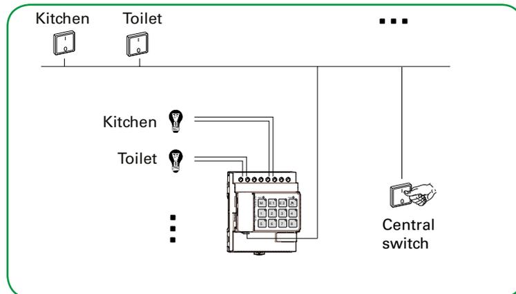
Dimming, switching, blind and roller shutter each have a separate central object with a corresponding central object.
