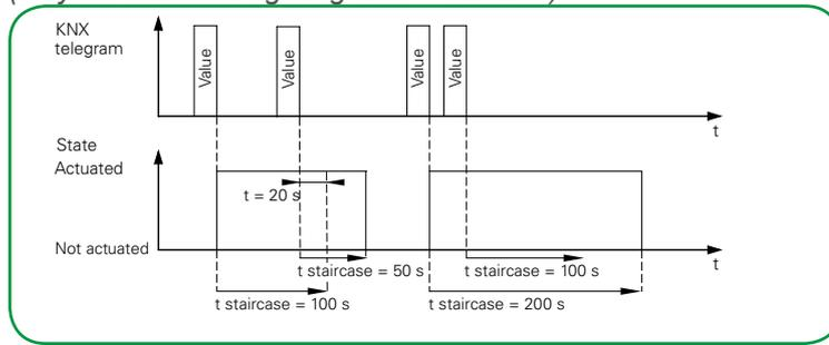
Once a new telegram has been received, the staircase lighting time is restarted with the higher value.
