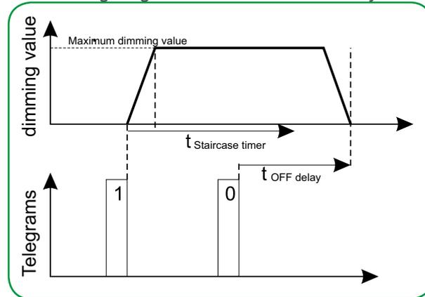
For staircase lighting time functions with *Manual switching off* and warnings activated, the staircase lighting time function is immediately deactivated with a warning when an "Off" telegram is received. The off-delay elapses. No warning is generated.
