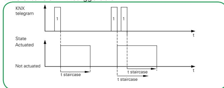
Once a new telegram with the object value "1" has been received, the staircase lighting time is restarted.
