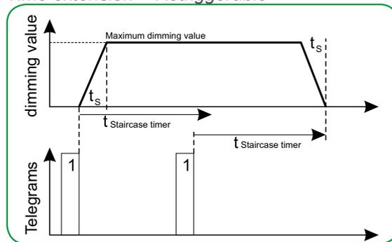
Once a new telegram with the object value "1" has been received, the staircase lighting time is restarted.
