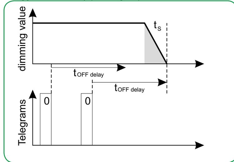
Moreover, for the off-delay, you can also select *Retriggerable and adding*. The delay time is added when the same telegram value is received, e.g. using a separate button. You can define the maximum number of additions.
