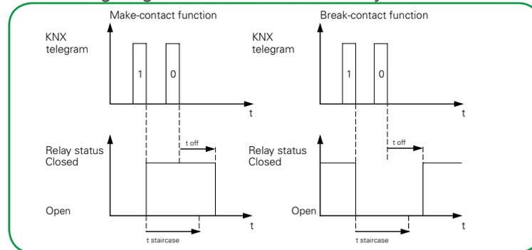
For staircase lighting time functions with *manual switching off* and warnings activated, the staircase lighting time function is immediately deactivated with a warning when an “Off” telegram is received. The off-delay elapses. No warning is generated.
