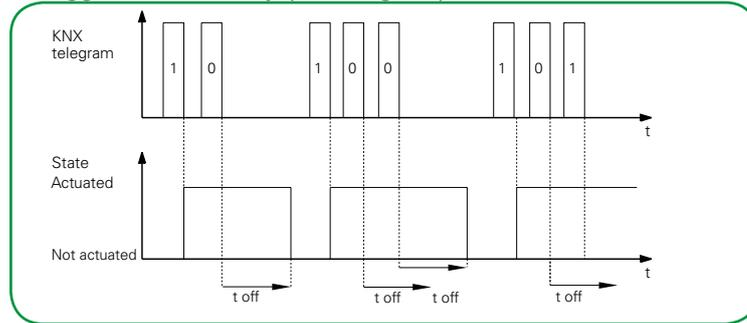
Moreover, for the off-delay, you can also select *Retriggerable and adding*. The delay time is added when the same telegram value is received, e.g. using a separate button. You can define the maximum number of additions.
