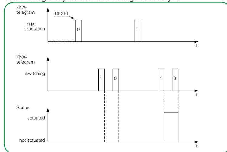
The parameter setting causes the “logic object” to be set to the value “0”. After a RESET, the actuator does not switch the output until a “1” telegram has been received on the “logic object”.
