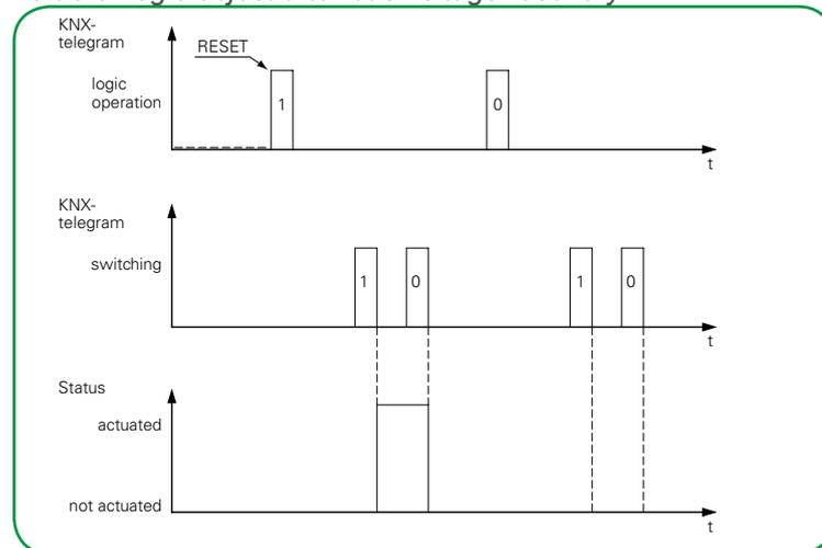
The logic object is preset with the value “1” after a RESET (bus voltage recovery and download). This enables switching to be carried out as usual using the switch object. The power-on lock is not active until a “0” telegram has been received via the logic object.
