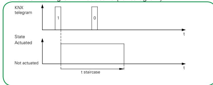
A telegram with the object value 0 has no effect. The set staircase light time continues to run normally until the end.
