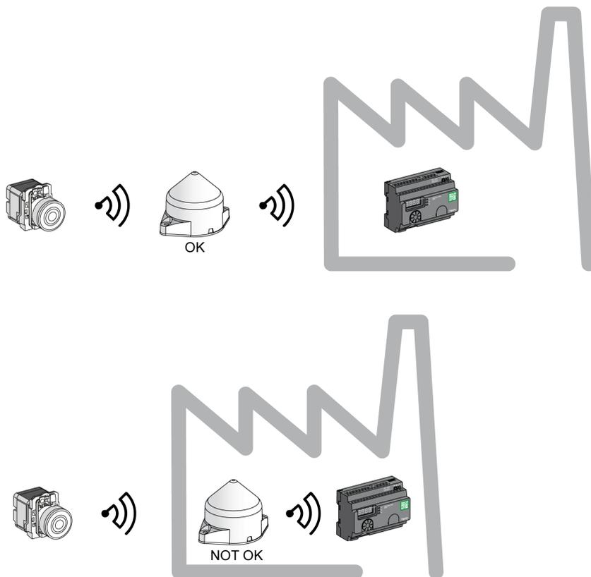
**NOTE:** In this case, if there is no relay antenna, the signal received by Harmony Hub may not be sufficient.
