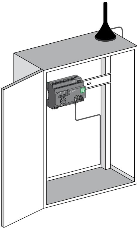
The antenna is equipped with a magnet at the bottom to mount it on the metal cabinet.
