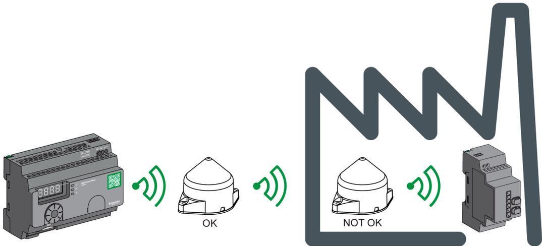
**NOTE:** The antenna should be placed before the obstacle. The signal will be amplified before the obstacle to enable to go through it.
