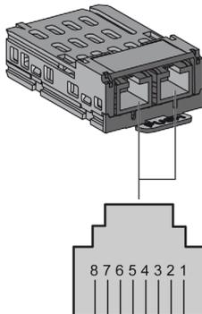
The following table shows the pin details of the RJ45 connector:
