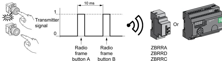
ZBRT1 is used for applications where single pulse is required (for example, remote start of machine and reset after machine fault detection).
