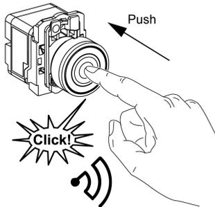
The radio message is sent when the button is pressed, signaled by a click. If the button is held down, the message is not transmitted continuously. The message is not sent when the button is released.
