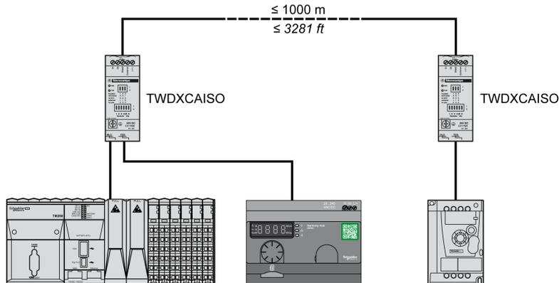
For distances longer than 20 m (65.62 ft), verify that the other devices connected to the bus are isolated. If other devices are not isolated, use the TWDXCAISO module.
