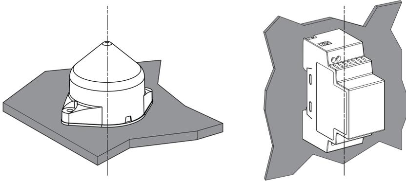
The antenna and the receiver are installed following their vertical axis.
