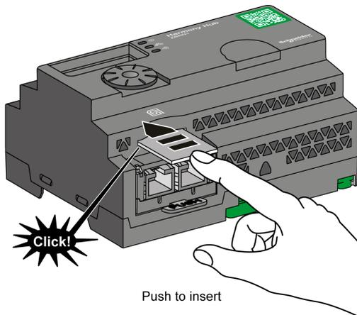
Push to insert the SD card into the SD card slot on Harmony Hub. Make sure that the SD card is inserted properly.
