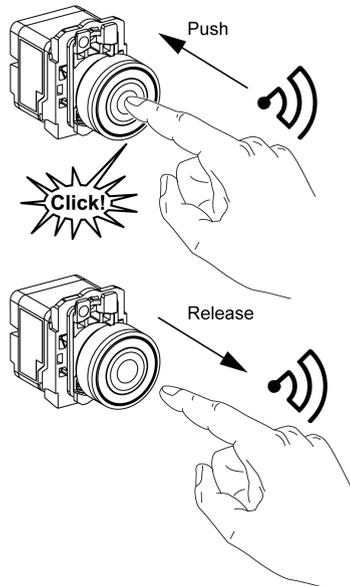
The radio message is sent when the button is pressed, signaled by a click.
