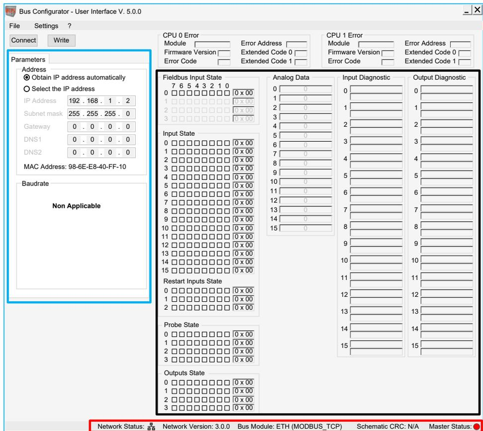
At the top right there are the boxes **CPU Error 0** and **CPU Error 1**, which display the diagnostic information if the Modular Safety Controller detects an error.
