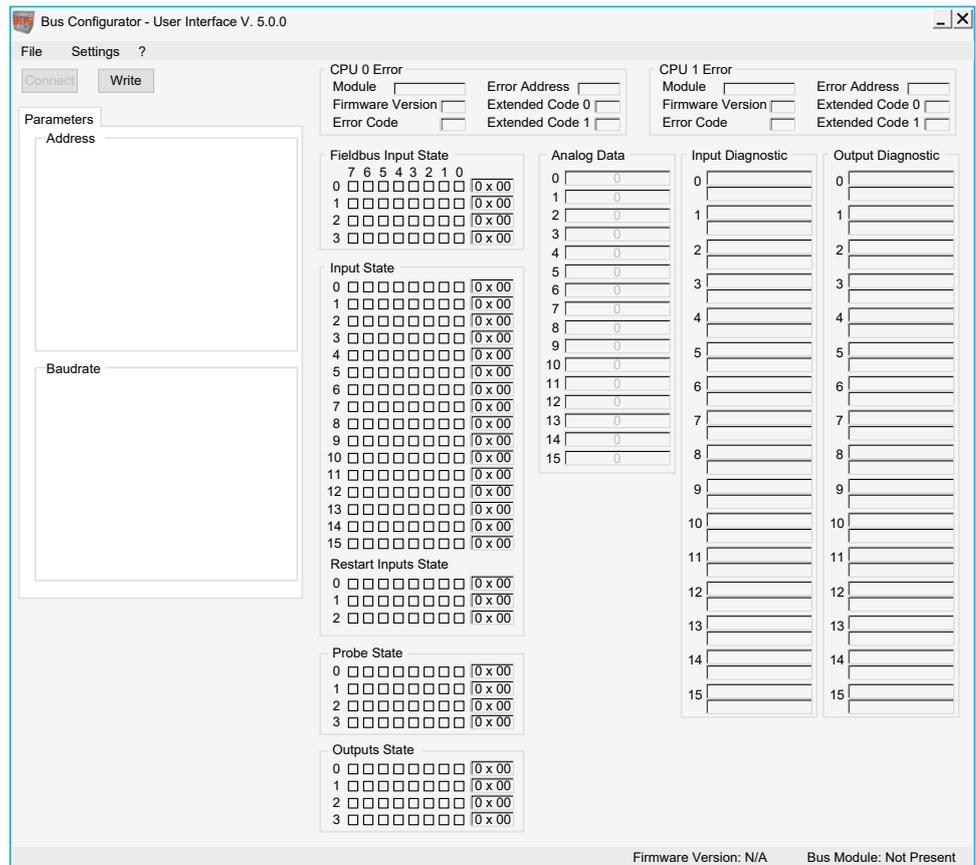
**NOTE:** When **Connect** button is not available, the **Bus Module** label at the bottom right shows the module as **Not Present**.
