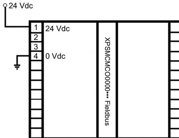
**NOTE:** Use a fuse on the incoming 24 Vdc power, sized appropriately for the requirements of the module.
