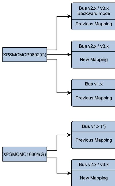
\* This combination is available when the XPSMCMC10804(G) application does not exceed the XPSMCMCP0802(G) application capabilities (for example, does not use more than 8 safety-related function blocks or 16 fieldbus probe function blocks or 8 fieldbus inputs function blocks).
