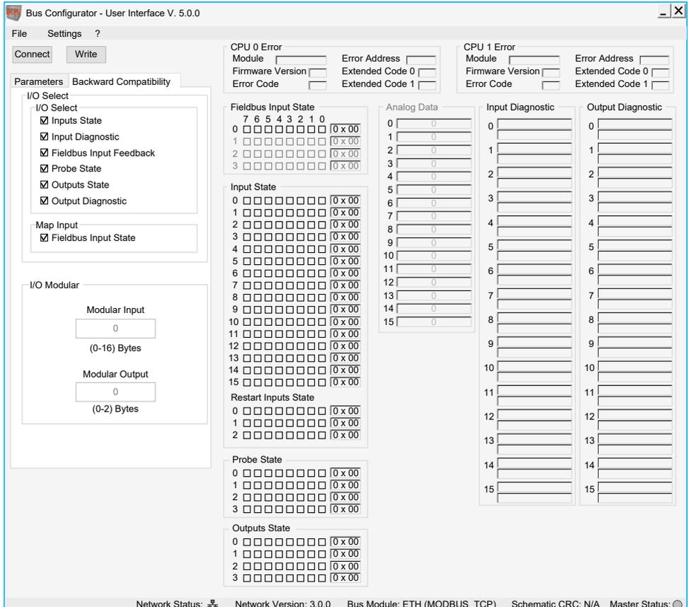
When the configuration data are set, press the **Write** button to send them to the module.
