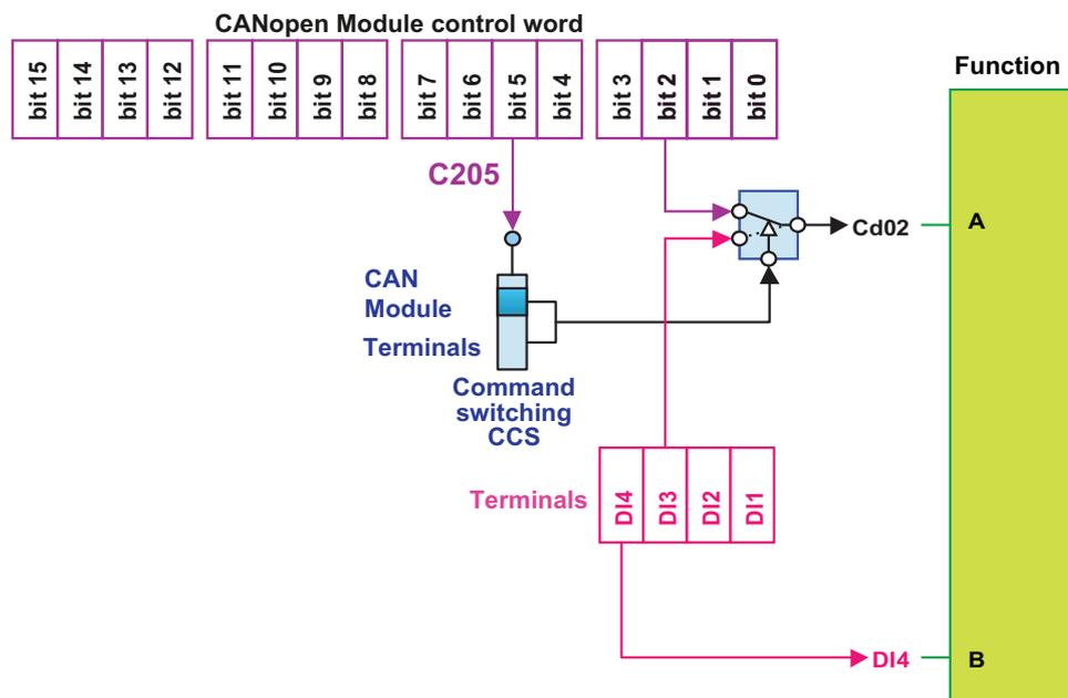
When a function is assigned to a switched bit (Cd00 to Cd15), the function can be activated via Terminals or selected communication channel according to the active command channel. To switch between Terminals and communication modules, use **[Command Switching]** function.
