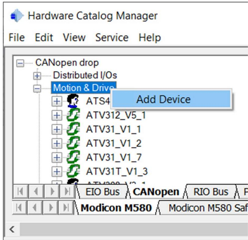
Once imported, you should see the soft starter in the **Motion & Drive** section. The two topics **default** and **PDOs only** are used in the CANopen device configuration screen of EcoStruxure Control Expert to select which objects are mapped and linked to an application variable.
