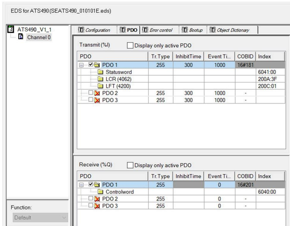
PDOs are linked to the %Mw variables, the mapping is automatically generated by EcoStructure Control Expert according to the index defined in the controller configuration panel and to the PDOs and to the device Node ID.
