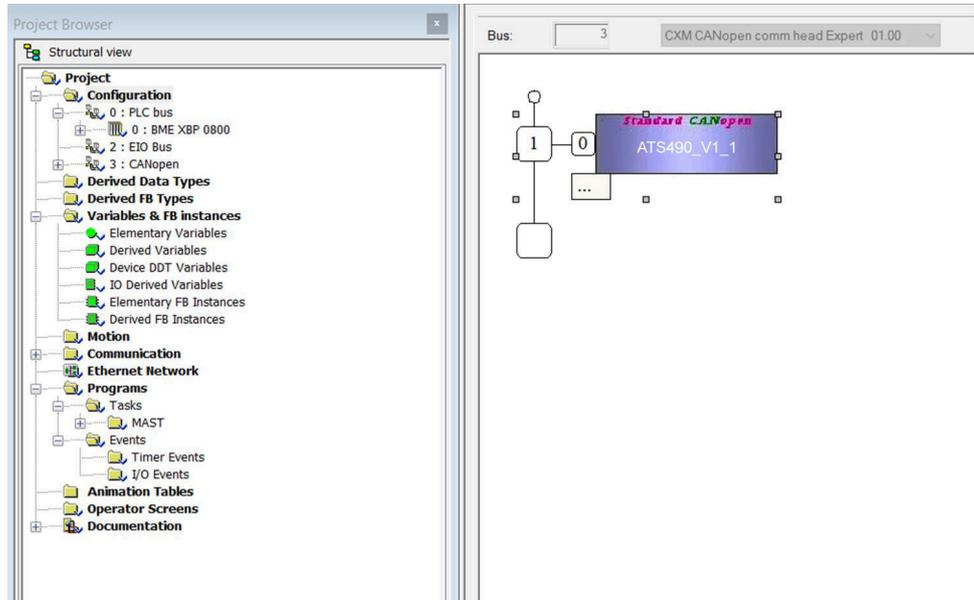
In the example below, TPDO1 and RPDO1 are selected which provides the basic control command of the soft starter with the Standard mode profile.
