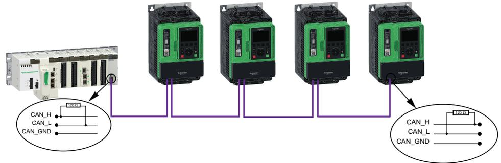
**NOTE:** A 120 ohm terminating resistor between CAN\_L and CAN\_H is used for this purpose.
