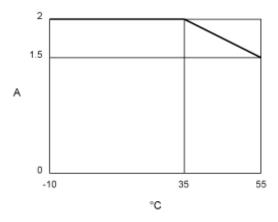
If the dissipation restriction of adjacent modules is not possible in your configuration, the de-rating must shift by -5 °C (- 9 °F), and 2 A / output can be maintained at 30 °C (86 °F). In most industrial applications, this would require the module to be in an air conditioned enclosure to maintain such temperatures.
