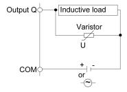
In applications where the inductive load is switched on and off frequently and/or rapidly, ensure that the continuous energy rating (J) of the varistor exceeds the peak load energy by 20 % or more.
