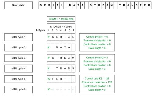
The process of preparing and splitting up the transmission data is the same, regardless of whether the *Block Forward* mechanism is used:
