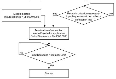
The following figure shows the synchronization procedure using the *InputSequence* and *OutputSequence* registers.
