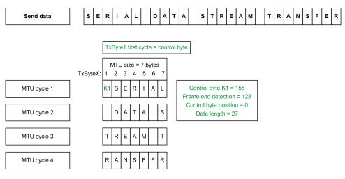
In contrast to the figure in Transmit Data: Preparation of the Cyclic Data, Maximum Organization, and Monitoring of the Individual Steps, page 125), this results in a saving of two MTU cycles for the same frame length and MTU size. A new frame can be started after the last MTU cycle 4.
