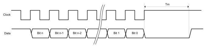
In the example 2 the **Monoflop check** parameter must be configured to low level so that the clock generation is postponed until the data line goes low.
