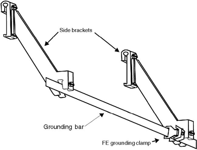
A technical diagram showing the components of the STB XSP 3000 kit. It features two side brackets, each with a circular hole at the top and a rectangular base. A long, thin grounding bar is positioned between them. One end of the bar is secured by an FE grounding clamp. Arrows point from the text labels 'Side brackets', 'Grounding bar', and 'FE grounding clamp' to their respective parts in the diagram. |
