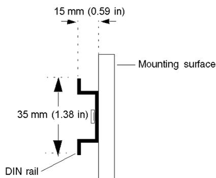
Select a DIN rail that is wider than the cumulative widths of modules you will install on it. In this example, select a DIN rail that is at least 152 mm (6 in) long.
