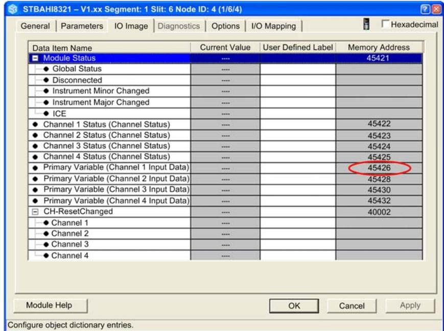
In the above example, the **Alignment** parameter is not enabled. Input data begins at memory address 45426. Because 45426 is an even number, input data begins at a 32-bit boundary. In this case, it is not necessary to enable the **Alignment** parameter.
