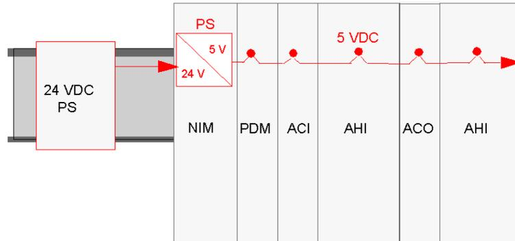
The NIM can supply maximum current of 1.2 A to the island segment modules. If your island design requires more power than the NIM can provide, you can:
