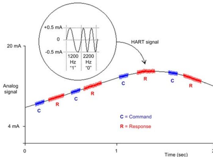
These digital signal frequencies are higher than the analog signaling frequency range of 0...10 Hz. The digital signal is typically isolated using a passive high-pass filter with a cut-off frequency in the range of 400 Hz to 800 Hz. The analog signal is likewise isolated using a passive low-pass filter.
