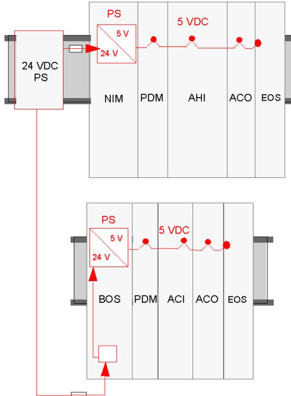
Operating voltages for the island range from 19.2 Vdc to 30 Vdc.
