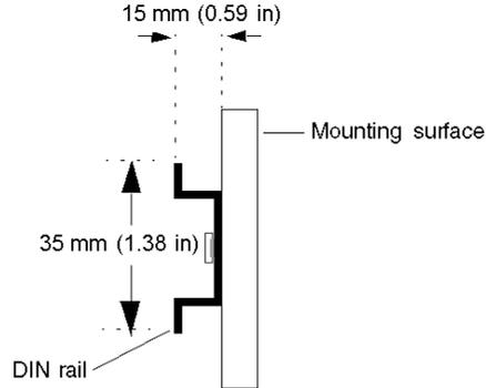
Use M5 threaded mounting hardware to affix the DIN rail to the mounting surface. Allow a maximum spacing of 150 mm (5.91 in) between each mounting hardware.
