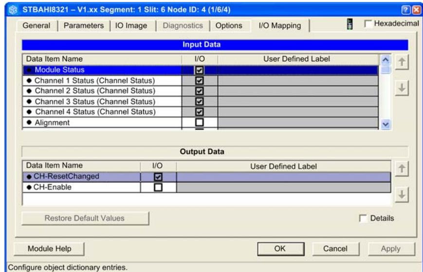
**NOTE:** Configuration changes entered in this tab take effect only after you use the Advantys configuration software to:
