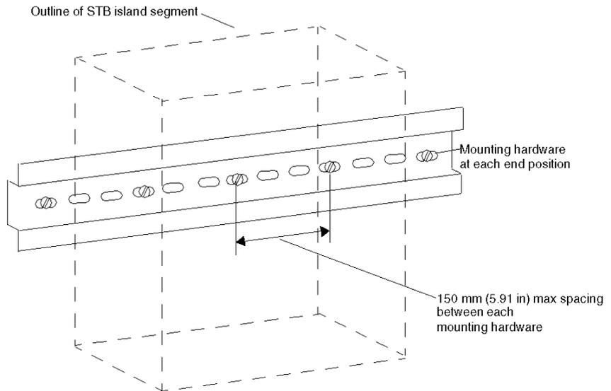
Low profile 7.5 mm (0.30 in) deep DIN mounting rail can be used with low profile mounting hardware such as flat head screws, with countersunk mounting holes.
