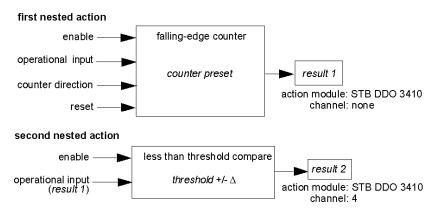
Result 2 (from the compare block) is the result that the nested reflex action will send to an actual output. Because the result of a compare block needs to be mapped to a digital action module, result 2 is mapped to channel 4 on an STB DDO 3410 digital output module.
