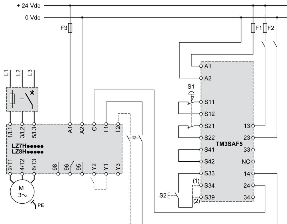
**S1** Emergency STOP button with two NC contacts, Harmony XB4 or Preventa XCS safety limit switches
