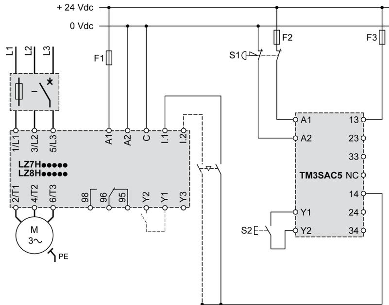
**S1** Emergency stop button with two NC contacts, Harmony XB4 or safety limit switches Preventa XCS.
