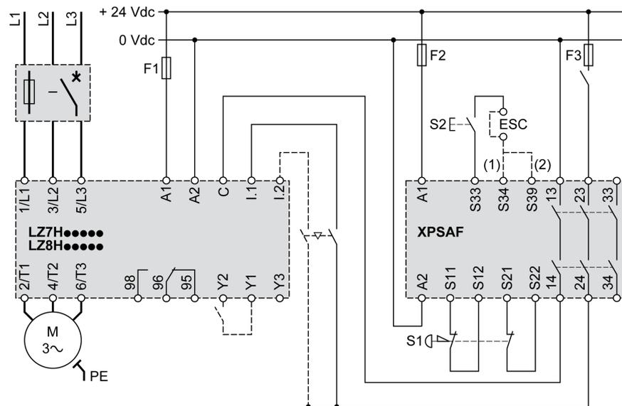
**S1** Emergency STOP pushbutton with two NC contacts
