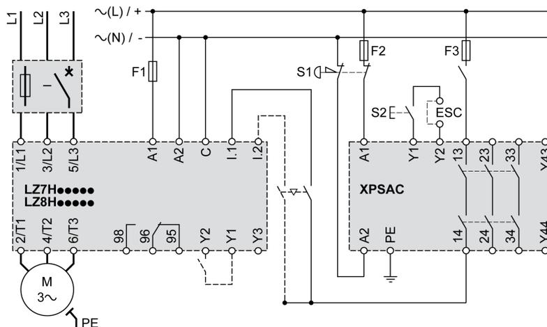
**S1** Emergency STOP pushbutton with two NC contacts
