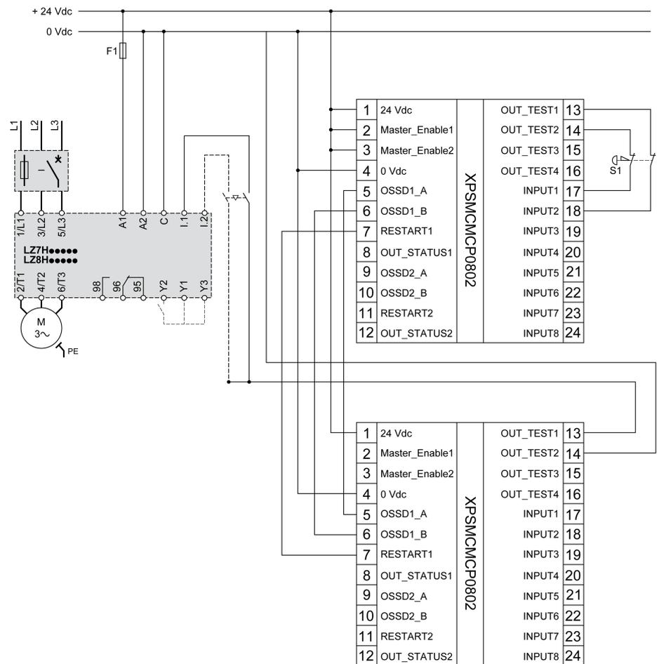
**Dual-Channel and Extended XPSMCM Modular Safety Controller - Cat.4, PLE According to EN ISO 13849:2006 and SIL 3 According to EN IEC 62061:2005**
