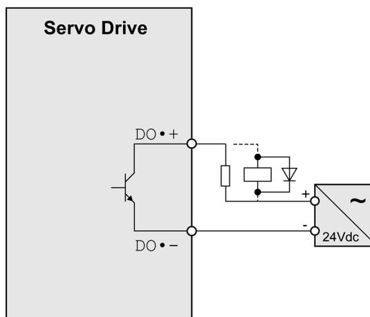
Example of digital output OCZ with internal power supply (negative logic):
