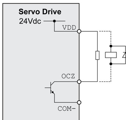
Example of digital output OCZ with external power supply (negative logic):
