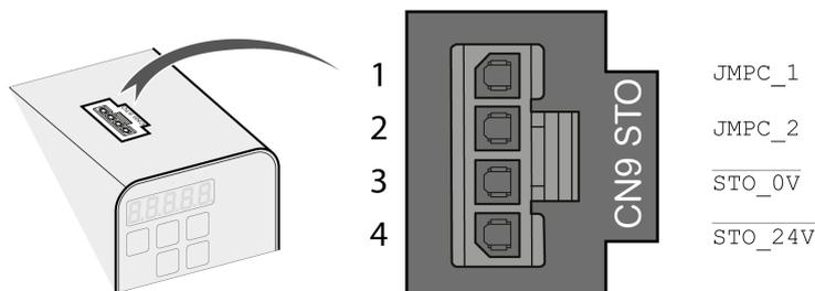
The STO interface (CN9) is a 4-pin female connector. The following table describes the contacts of the connector:
