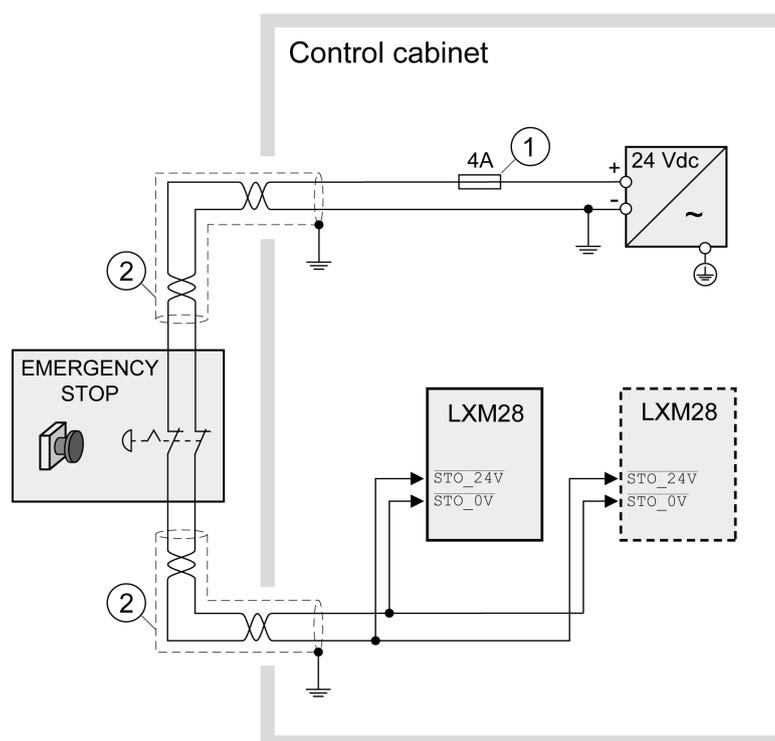
**1** If the maximum output current of the 24 V power supply exceeds 4 A, a 4 A slow-blow fuse is required.
