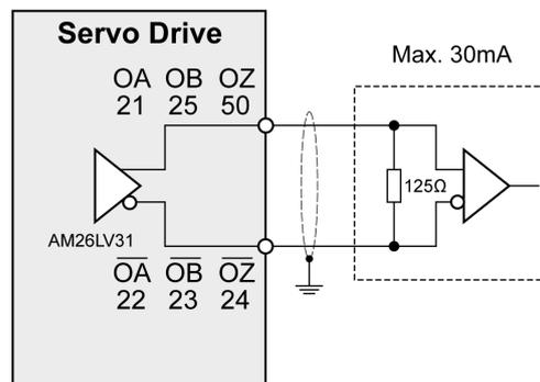
Example of encoder output signal, high-speed optocoupler.
