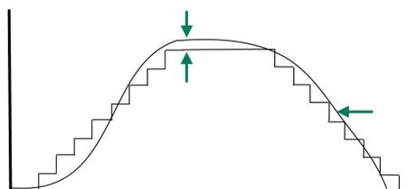
Increasing *P8-28* (GEARFILTT2) and *P8-29* (GEARFILTVELFF) compensate the delay, but adds overshoots.
