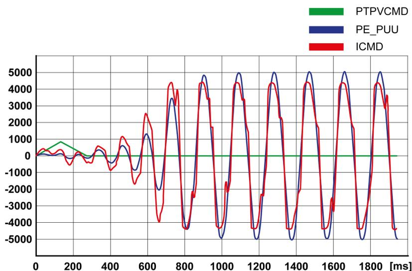
**NOTE:** The process of tuning requires trials of successive approximations. Values that are too high or too low relative to the other relevant values might cause instability. If it is necessary to have a low or high value of the parameter in the preceding example, you may need to adjust the values of the other relevant parameters to compensate and achieve a stable system.
