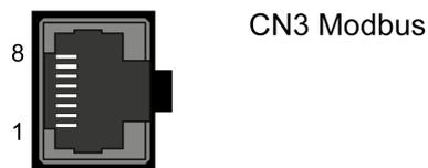
The commissioning interface (CN3) is an RJ45 connector. The following table describes the contacts of the connector:
