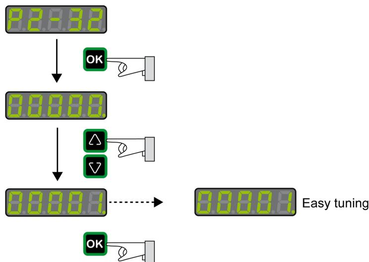
After you have started Easy Tuning via P2-32, the display of the HMI shows the progress as a percentage from `tn000` to `tn100`.
