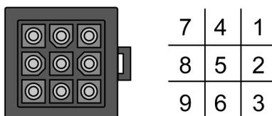
Encoder connection MIL connector (Type B), motor side:
