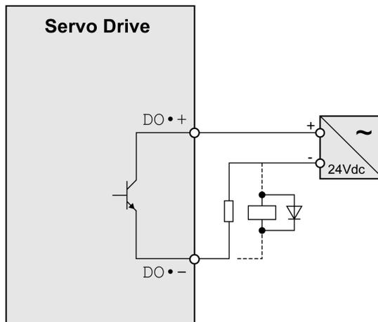
Inductive loads using DC voltages may damage the signal outputs. A protection circuit is required to protect the signal outputs against inductive loads.
