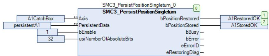
Finally, the POU of persisPositionAxis is called in Motion task to complete programming.
