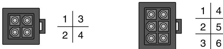
Motor connection MIL connector (type C and type D), motor side:
