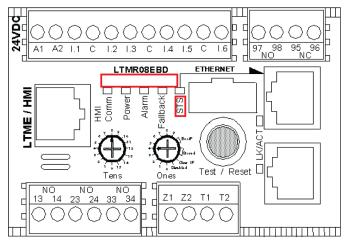
MBTCP+EIP Generation hardware is the latest implementation of the Ethernet based TeSys T product. It can be identified by the following characteristics:
