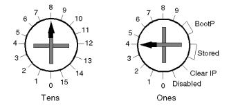
The settings of the rotary switches determine the source of the LTMR controller's IP address parameters and the FDR service activation, as follows:
