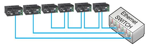
**NOTE:** To keep the integrity of Ethernet daisy chain network when one or more LTMR controllers are powered off, add an external permanent 24 Vdc power supply (not shown) to power the LTMR controller.
