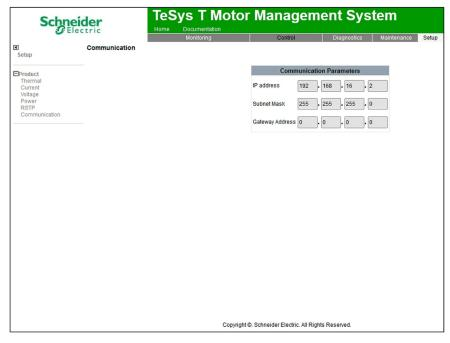
**NOTE:** This IP address is used only if the product is in stored IP mode, page 30. Restart the device in stored IP mode for the parameters in the page to take effect.
