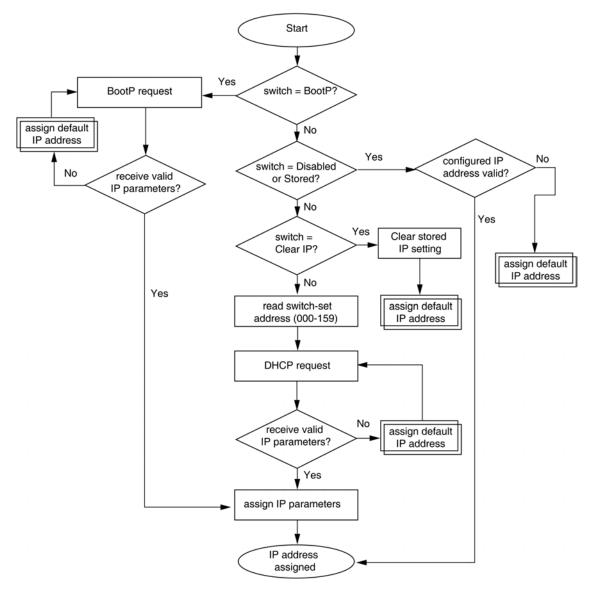
**NOTE:** The Fast Device Replacement (FDR) service is not available when the default IP parameters are used.
