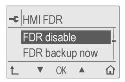
"FDR disable" is an option to deactivate the HMI FDR services in case the user wants to use LTMCUF as a basic LTMCU. By default, the HMI FDR services are enabled.
