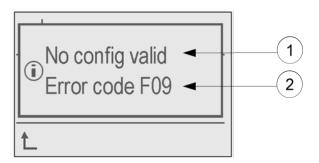
1 Trip/Alarm name Detected error Code
