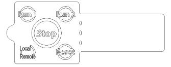
**NOTE:** The label must be chosen according to the LTMR controller's operating mode. The keys' label on the local control interface must be appropriate to the functions of the LTMR operating mode.
