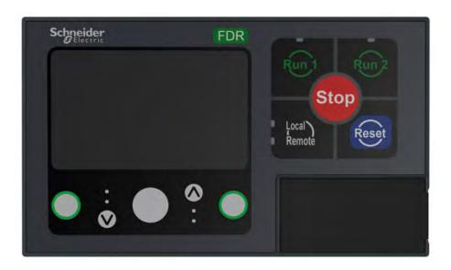
HMI FDR services facilitate operator task when replacing a drawer in a high continuity of service environment, without needing a computer nor expertise in configuring LTMR
