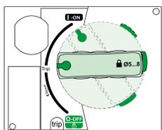
The device has tripped on electrical fault, the rotary handle has moved from the **I (ON)** position to the **Trip** position.
