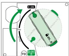
To close the device, turn the rotary handle clockwise from the **O (OFF)** position to the **I (ON)** position.
