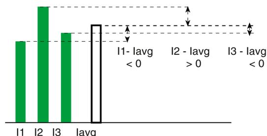
If the maximum current unbalance value is higher than the phase unbalance protection lunbal pickup, the tunbal time delay is actuated.
