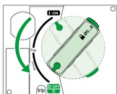
To open the device, turn the rotary handle counterclockwise from the **I (ON)** position to the **O (OFF)** position.
