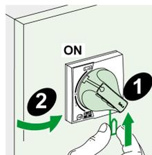
It is possible to temporarily disable this lock to open the door when the device is in the I (ON) position.
