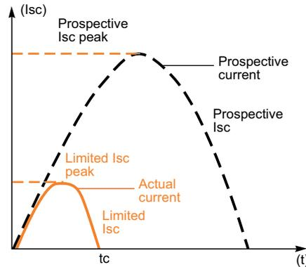
The exceptional limiting capacity of TeSys GV5 / GV6 devices is due to the rotating double-break technique (very rapid natural repulsion of contacts and the appearance of two arc voltages in-series with a very steep wave front).
