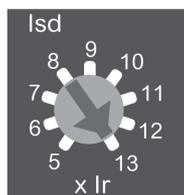
The short-time protection pickup I<sub>sd</sub> is set by using a multi-position dial.
