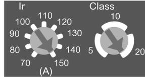
The long-time protection is set by two dials according to the starting characteristics of the application.
