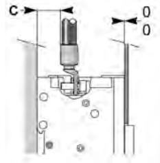
A rear insulation screen or long terminal shield is required if the distance C is less than 8 mm (0.32 in).
