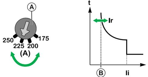
The values of  $I_r$  are adjustable from 0.7 to 1 x  $I_n$  (circuit breaker rating) as shown in the following table:
