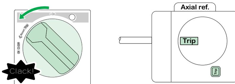
After a trip, reset a circuit breaker with a side rotary handle in the same way as for a circuit breaker with an extended rotary handle, page 55.
