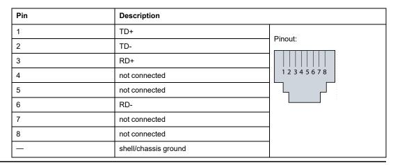
**NOTE:** The TD pins (pins 1 and 2) and the RD pins (pins 3 and 6) can be reversed to allow the exclusive use of straight-through cables.
