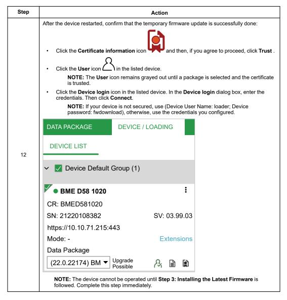
**NOTE:** Do not login or connect EcoStruxure Automation Expert to the Modicon M580 distributed PAC until all installation steps are completed.
