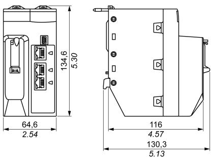
**NOTE:** Consider the height of the controller when you are planning the installation of the local backplane. The controller extends below the lower edge of the backplane by:
