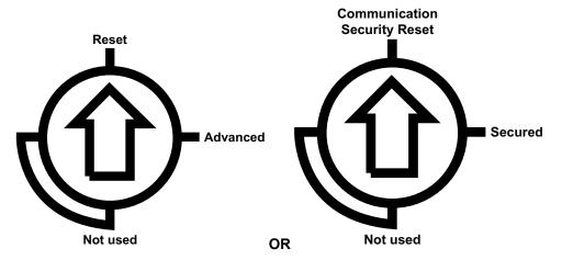
Use the screwdriver to select a rotary switch position according to the table below:
