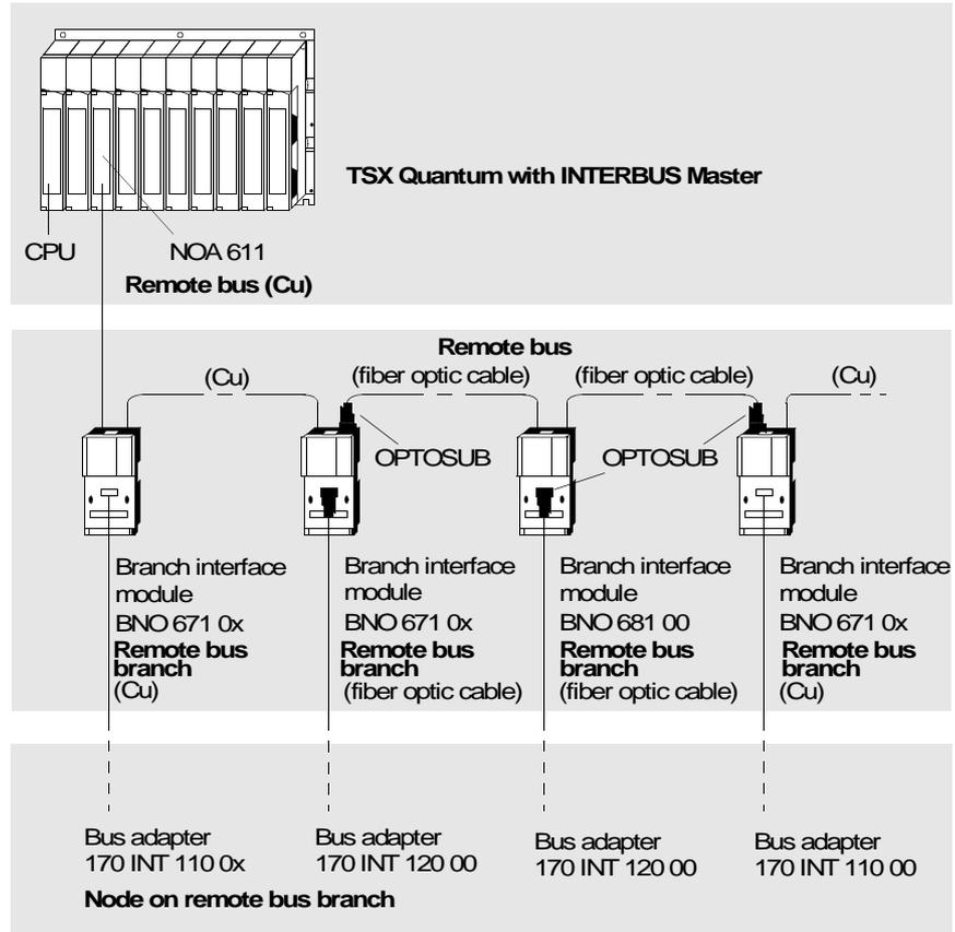
The conversion from copper cable to fiber optic cable is done with OPTOSUB or OPTOSUB PLUS, depending on the module used (see section *Transition from copper cable ↔ fiber optic cable*, p. 12).
