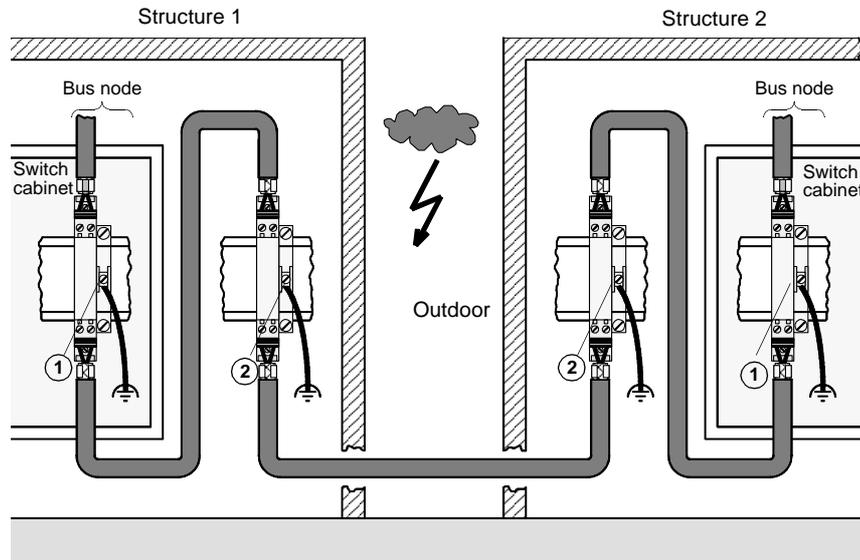
Type and number of the lightning arrestors from Dehn und Söhne GmbH & Co KG for a remote bus cable LiYCY (INTERBUS):
