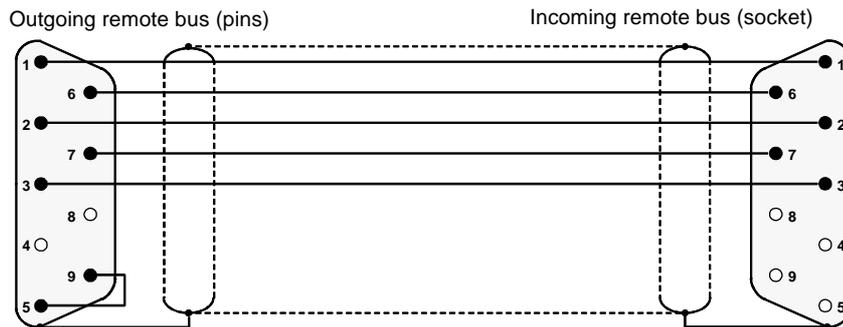
**Pin configuration of the outgoing remote bus**
