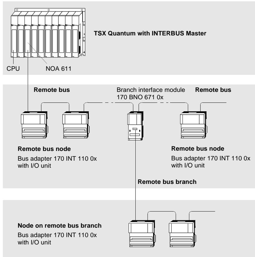
**Cable type: Fiber Optic Cable** This example shows the structure of an INTERBUS configuration with Momentum I/O modules using fiber optic cable.
