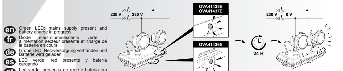
**en** Green LED: mains supply present and battery charge in progress
