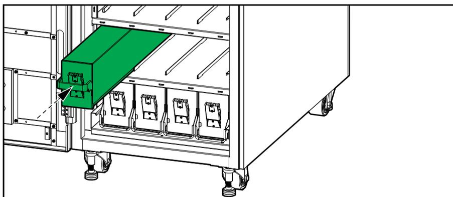
3. Fasten the battery modules with a screw in front of the battery module
