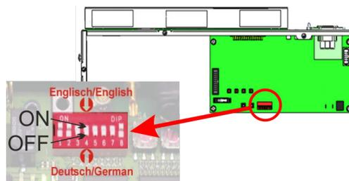
The system can communicate in "German" and "English". "German" is pre-set by the manufacturer but can be changed to "English" via a DIP switch (Fig. 23). Proceed as follows to make the changeover:
