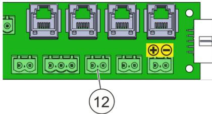
Fig. 39: Connecting terminal "Manual call point"
