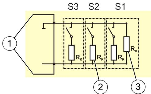
Fig. 40: Manual call points parallel connected
