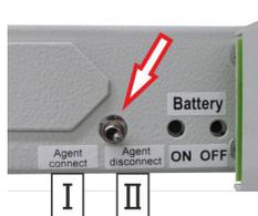
Fig. 26: Blocking switch
