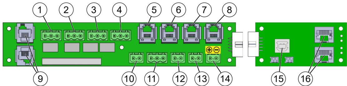
Fig. 7: "AT3 connection technology" card (left) and "NW network interface" card (right)
