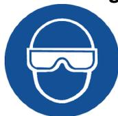
Protective goggles cover the entire area of the eyes (including the sides) and are used to protect the eyes from the extinguishing agent and from particles that are whirled up by the extinguishing agent.
