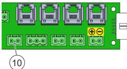
Fig. 11: Connection of external alarm device
