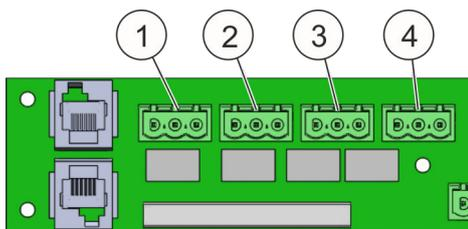
The system has four potential-free relay outputs (Fig. 8/1 to 4) each with one changeover contact.
