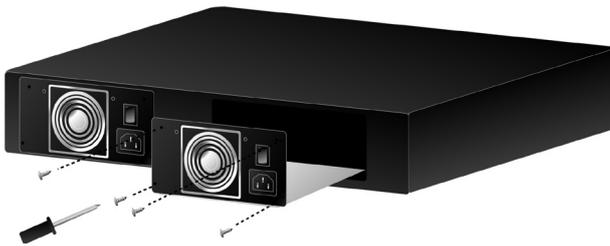
Figure 2. Install and remove the redundant power supply unit
