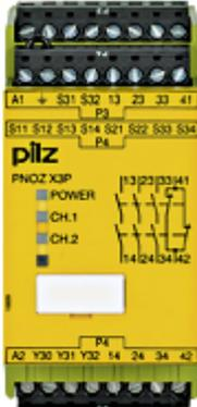
Safety relay (standalone) Inputs: 1-/2-channel wiring with/without detection of shorts across contacts Outputs: 3 N/O, 1 N/C, 1 semiconductor. Automatic/monitored start UB 24 - 240 V AC/DC, width: 45 mm, plug-in terminals of screw type Monitoring E-STOP, safety gates.
