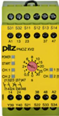
Safety relay (standalone) Inputs: 1- / 2-channel wiring with detection of shorts across contacts Outputs: 2 N/O, 2 N/O delayed UB 24 V DC, width: 45 mm, plug-in terminals of screw type Monitoring E-STOP, safety gates with 2 delay-on de-energisation contacts. Release time 12 stages from 0 - 30 s.
