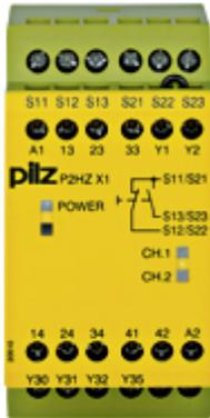
Safety relay (standalone) Inputs: 1 N/O, 1 N/C per pushbutton Outputs: 3 N/O, 1 N/C, 2 semiconductor UB 24 V DC, width: 45 mm, plug-in terminals of screw type Two-hand control device, monitoring the simultaneity of a two-hand pushbutton.
