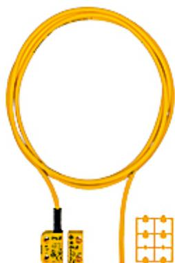
RFID safety switch 2 safe semiconductor outputs, connection cable 5 m, one direction of actuation IP6K9K, operating distance 11 mm, Sao = 8 mm, Sar = 20 mm; PU = 1 piece coded switch with actuator.
