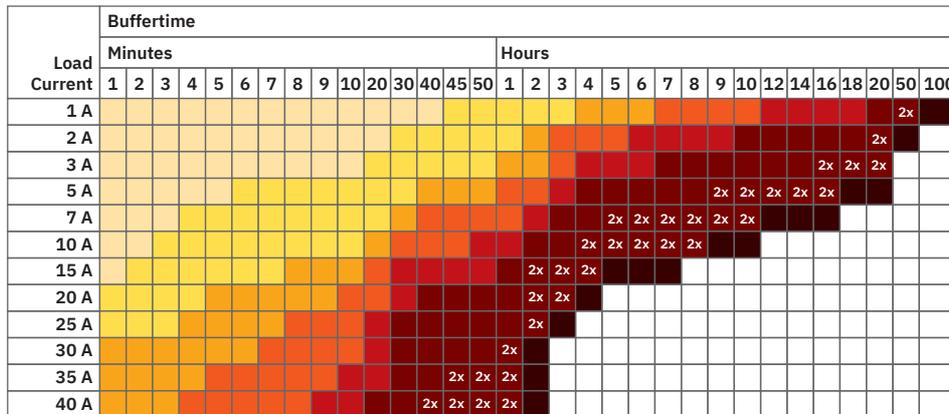
2x: In this case, two battery modules of the same capacity are required. The data is based on an ambient temperature of +25 °C at the start of use.
