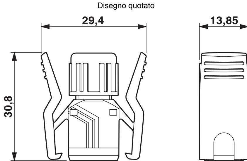
Custodia mobile RJ45, IP20, tornita
