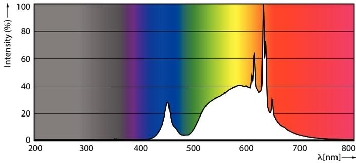
Spectral Power Distribution Colour - MAS LEDspot UE 2.1-50W GU10 DIM
