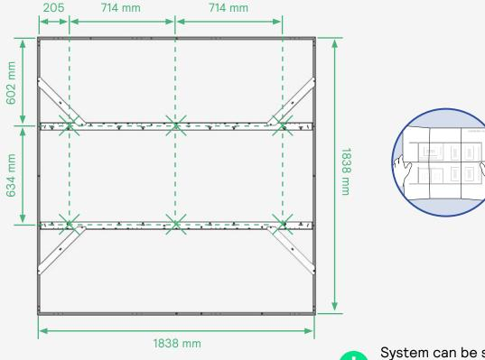
System can be suspended with steel cables with proper workload or threaded rods.
