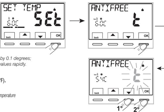
**i** Every time the ▲ or ▼ keys are pressed, it changes by 0.1 degrees; pressing and holding enables you to scroll through the values rapidly.
