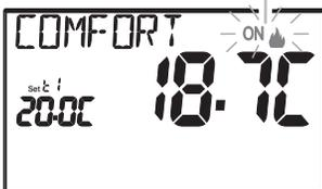
The thermostat is operative, displaying: Winter «heating» mode, the temperature Set at 20°C COMFORT, room temperature detected.
