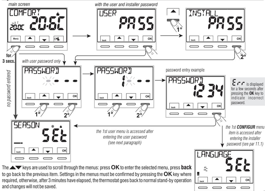
The ▲▼ keys are used to scroll through the menus: press **OK** to enter the selected menu, press **back** to go back to the previous item. Settings in the menus must be confirmed by pressing the **OK** key where required, otherwise, after 3 minutes have elapsed, the thermostat goes back to normal stand-by operation and changes will not be saved.
