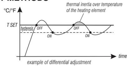
**As opposed** to the thermal differential, the temperature can be adjusted **MODULATING PROPORTIONALLY (PROP)** setting cycles from 7 to 20 minutes (default 10 minutes).
