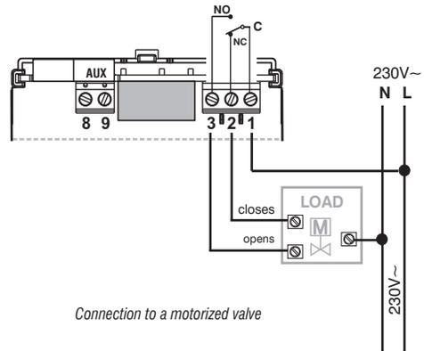
**N.B.:** with heavy inductive loads (pumps and solenoid valves), connecting an RC filter parallel to the load is recommendable.
