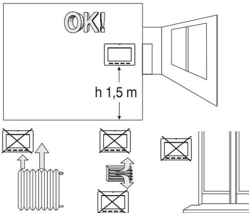
Install the thermostat preferably at a height of 1.50 to 1.60 m from the floor, far from sources of heat, air inlets, doors or windows and anything that may alter its operation.
