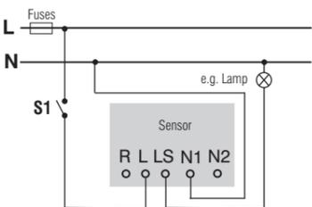
**Example: follow the wiring diagram below to connect two PIR Sensors to a single lamp:**
