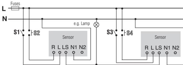
**Note:** it is possible to connect a pushbutton (S2, S4) to the sensor for manual operation.
