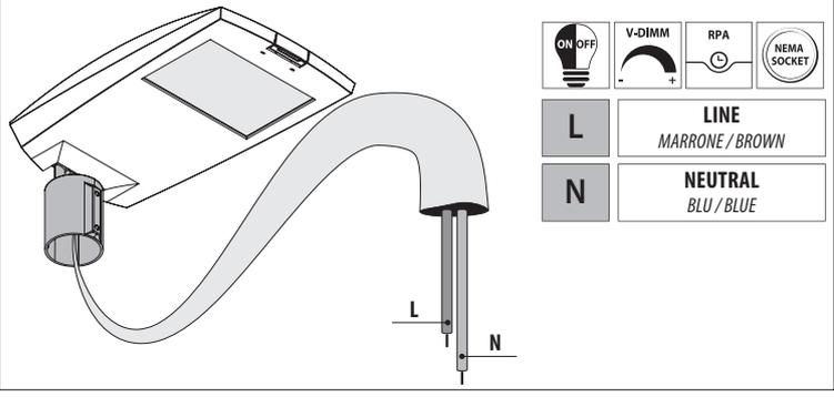
**3B ON/OFF WITH CONTROL PHASE WIRING**
