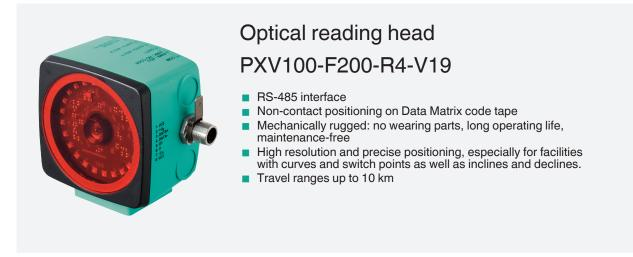
Read head for incident light positioning system
