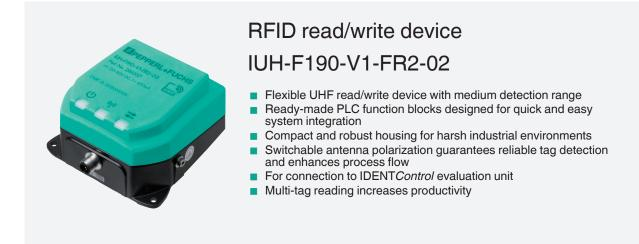
UHF RFID read/write device for IDENTControl, USA, Canada and Argentina
