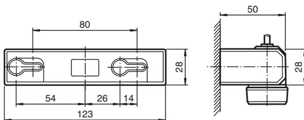
Mounting dimensions with mounting bracket set AIR30
