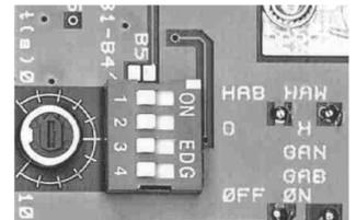
Use the potentiometer to the left of the switches to set the GAN and GAB times steplessly from 0.1 s ... 10 s.
