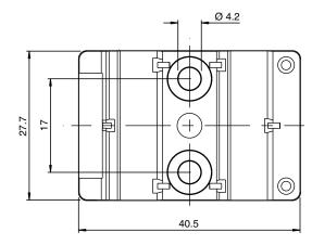
You may screw the device onto a level mounting surface using two M4 attachment screws. The attachement screws are not included.
