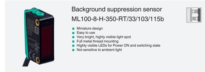
Triangulation sensor with background suppression, 350 mm adjustable detection range, red light, light/dark on, pnp output, fixed cable with M12 plug
