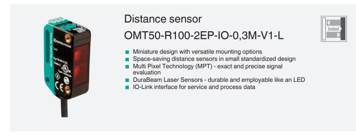
Measurement to object, 50 mm detection range, red laser light, laser class 1, measured value via IO-Link, 2 x push-pull output, fixed cable with M12 plug
