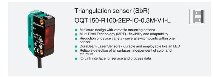
Switching diffuse mode sensor with measurement core technology, 150 mm detection range, red laser light, laser class 1, IO-Link, 2 x push-pull output, fixed cable with M12 plug
