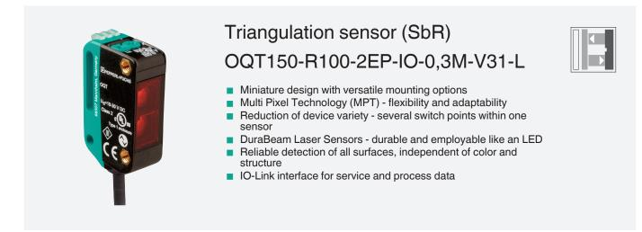
Switching diffuse mode sensor with measurement core technology, 150 mm detection range, red laser light, laser class 1, IO-Link, 2 x push-pull output, fixed cable with M8 plug
