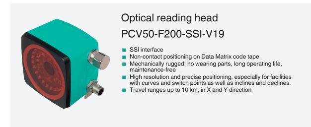
Read head for incident light positioning system
