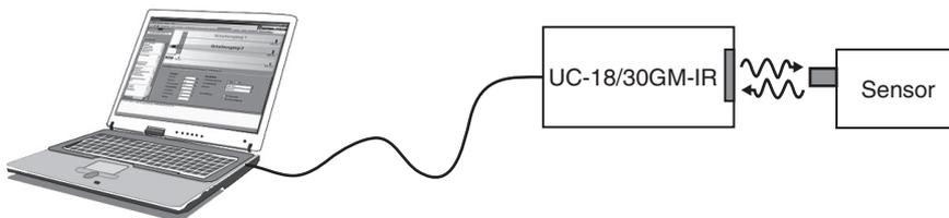
The ULTRA-PROG-IR parameterization software is also required for setting the sensor parameters. The ULTRA-PROG-IR software can be downloaded for free from the [www.pepperl-fuchs.com](http://www.pepperl-fuchs.com) website. The software allows all open parameters to be set, including:
