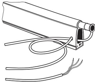
Insert the emitter and receiver into the hollow chamber.
