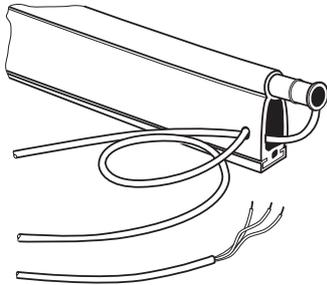
Slide the emitter and receiver into the upper chamber.
